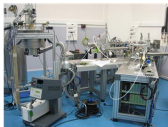
Two Beam-lines operating in vacuum 5 \times 10^{-8} mbars avoiding energy and current degradation
